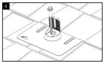
Insert lag bolt with EPDM backed washer through flashing. Tighten lag bolt until fully seated. FlashVue is now installed and ready for IronRidge XR Rails.
